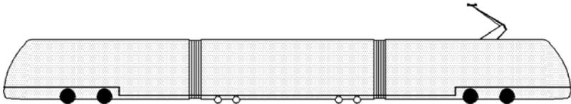
Fig. 1 – Partially low-floor tram with two axle running bogies
