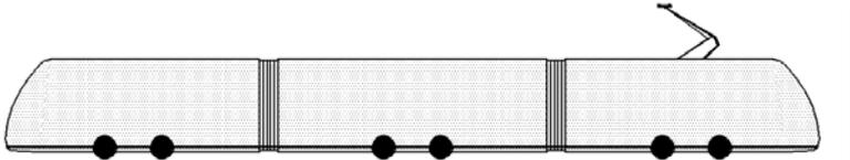
Fig. 2 – Fully low-floor tram with long carbody sections of the same length
