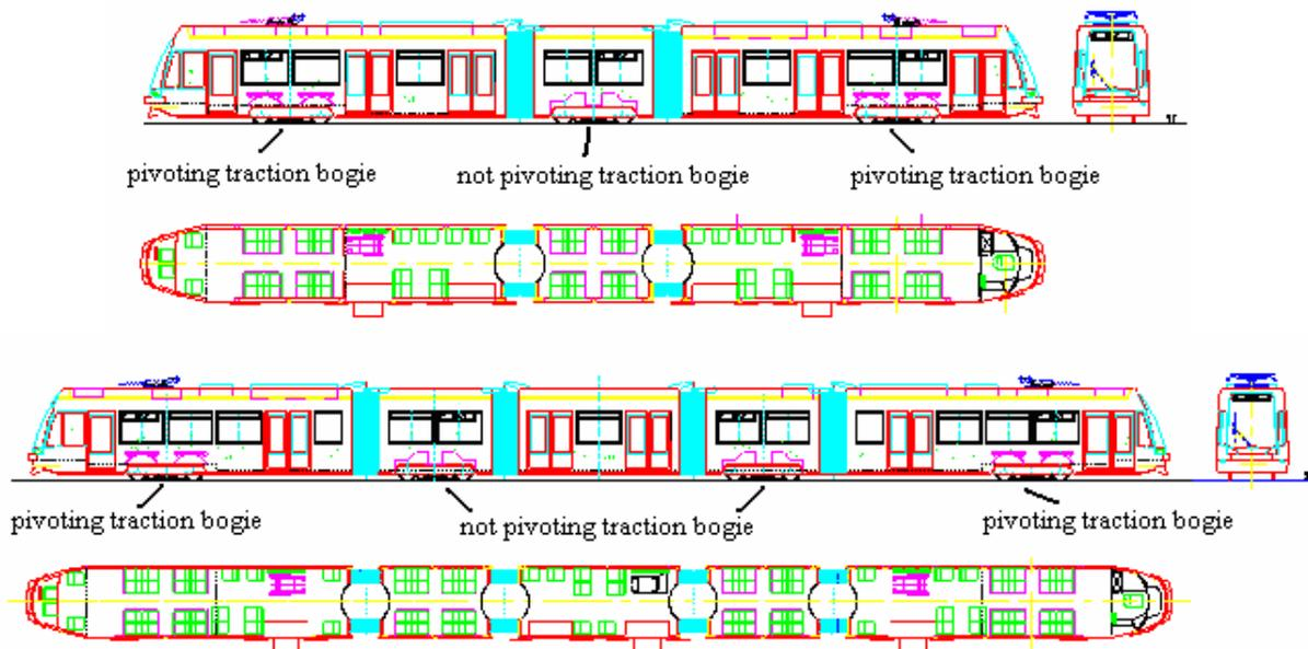
**Fig. 5 – Six-axle and eight-axle low-floor trams with short sections**
