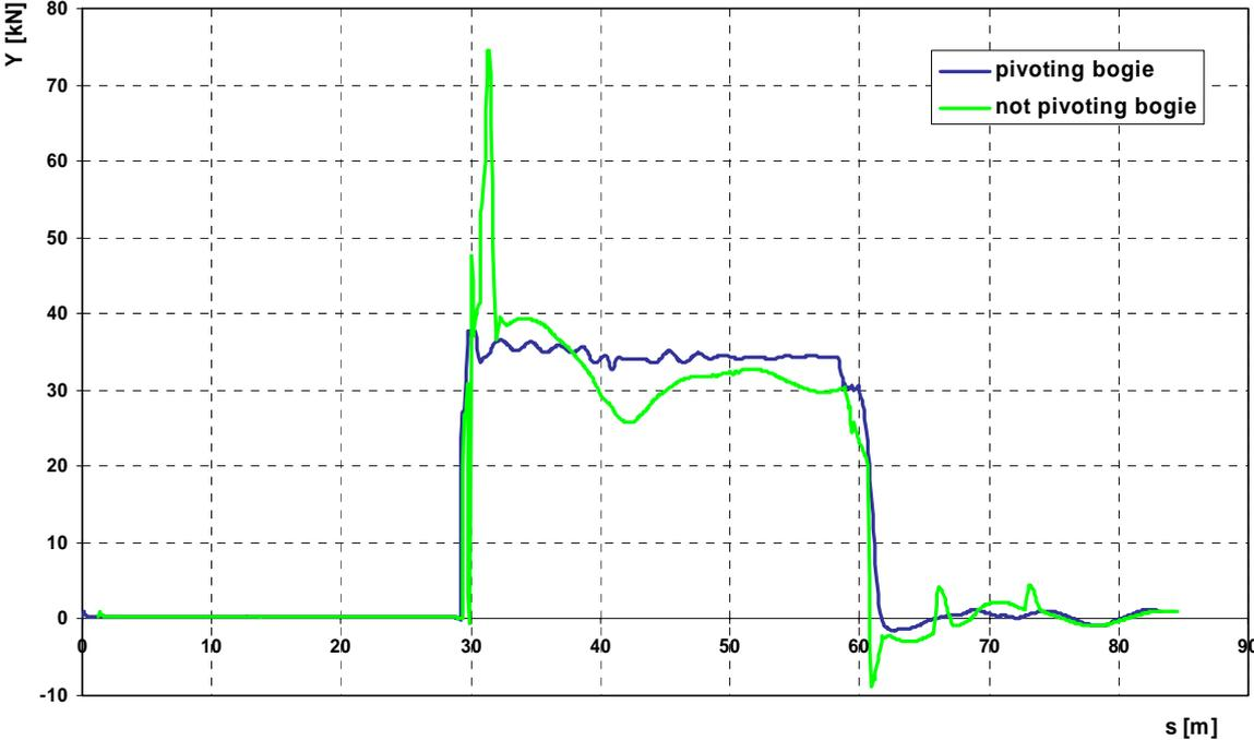
**Fig. 4 – Y forces on the outer wheel, first wheelset, speed 15 km/h, curve radius 20 m**
