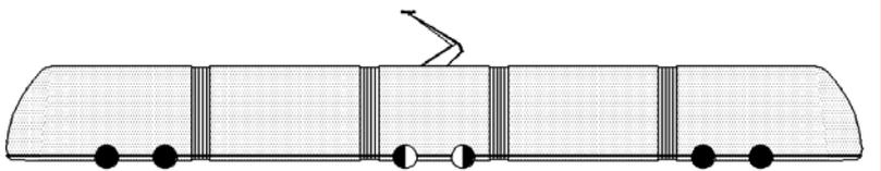
**Fig. 3 – Fully low-floor tram with short carbody sections and suspended long sections**
